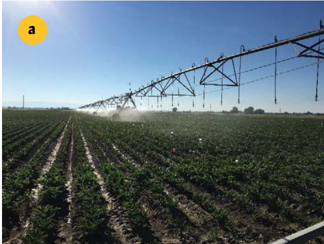
Figure 3. (a) GPS mounted variable rate sprinkler irrigation system and (b) sub-surface drip irrigation system at Powell Research and Extension Center can apply less water than furrow flood irrigation systems while meeting the crop water needs.
